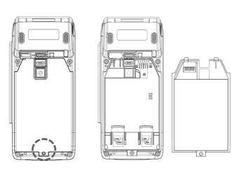
Identify the two SIM slots located in the bottom right corner inside the battery compartment.
