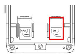
Now, insert a mini-SIM with the chip facing up, like the illustration. Close the battery compartment by placing the battery in its original space. Remember to re-install the screw.
